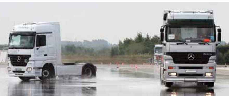
A Mercedes-Benz equipped with ESP (electronic stability program) with steering intervention on a wet split- \mu surface demonstrated a shorter braking distance and better control than a vehicle without it.
