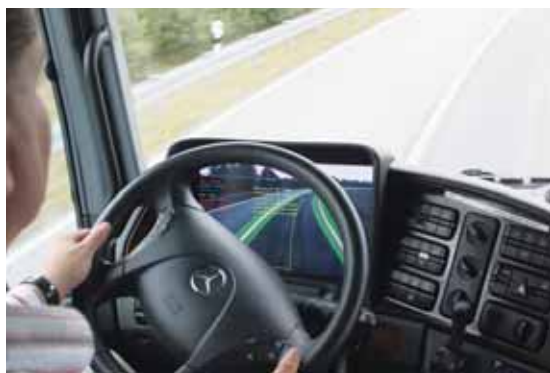
Torque applied from a servomotor can help drivers of commercial vehicles hold position in highway lanes.
