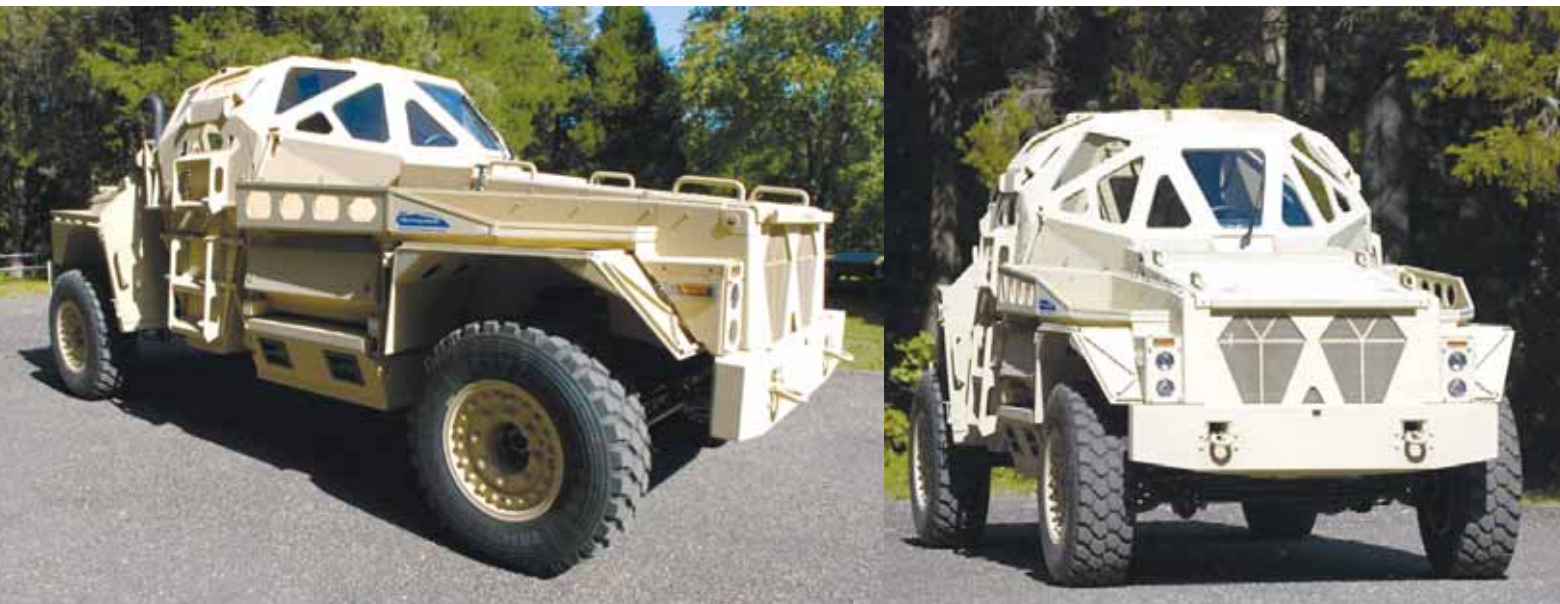
The ULTRA AP concept vehicle was developed by Georgia Tech Research Institute to illustrate potential technology options for improving survivability and mobility in future military combat vehicles.
