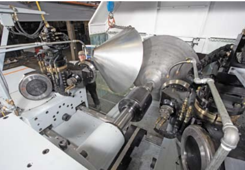
A part is removed after being spun during the machine's testing period.
