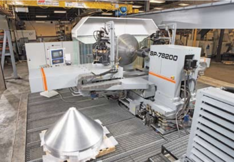
Glenn Metalcraft's new lathe features a 200-hp (150-kW) spindle, 100-hp (75-kW) hydraulic system and a three-station automatic turret.
