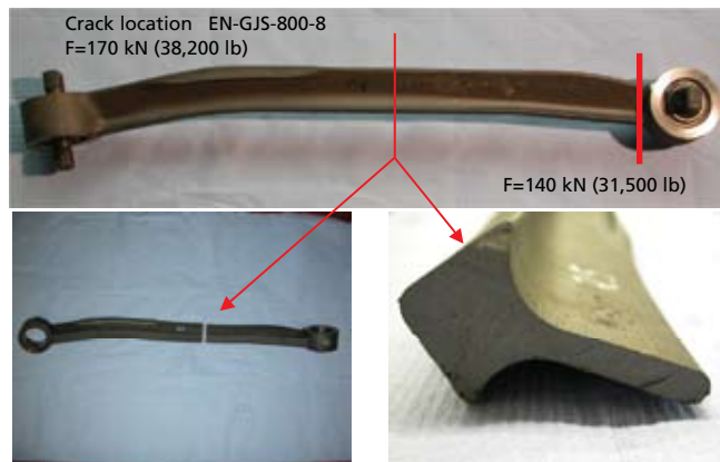
There were two areas where cracks initiated first in the fatigue tests with preloaded high-strength cast-iron suspension arms.
