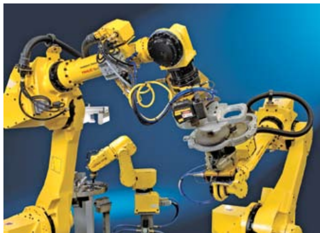
Two Fanuc robots can be deployed with a single controller.
