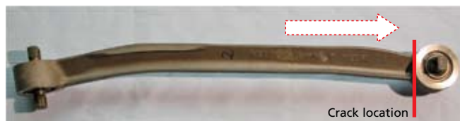
Researchers conducted constant and variable amplitude fatigue tests on suspension arms made from high-strength and ductile cast iron. The fatigue tests were performed on both un-preloaded and preloaded arms.
