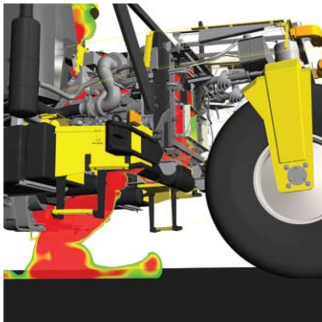
Exa's PowerCOOL is a tool that AGCO used to simulate thermal flow in the engine compartment. (Heat exchanger hidden to show effect.)
