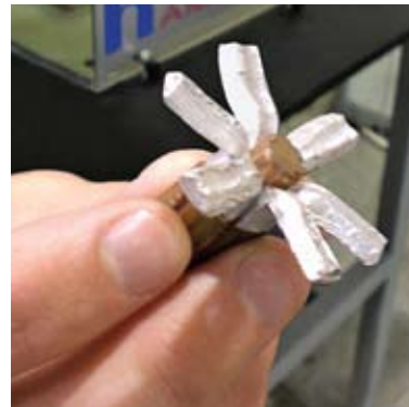
This aluminum-to-copper demonstration piece has been split apart to prove that the metals were bonded at a molecular level.
