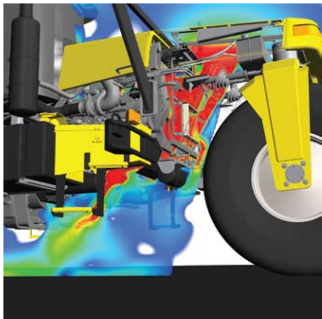
Exa's PowerFLOW simulation tool was used to analyze airflow movement. Flow is colored by velocity magnitude, with red the fastest and blue the slowest.
