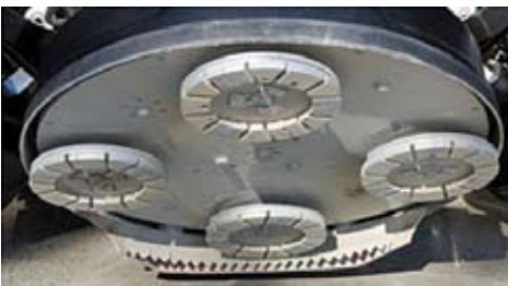
Three polishing heads (inset) let HTC's 2500 iXH finish about 500 yd 2 (418 m 2 ) of stone floor per day.
