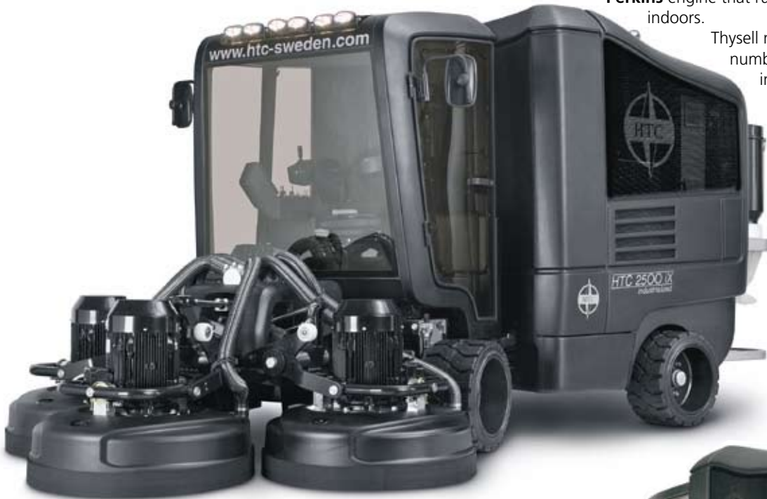
The system collects dust in three containers to meet environmental regulations.
