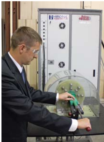
Michael Blakely places two dissimilar metals into Hirotec America's C3 machine for cold-welding by an electromagnetic pulse.
