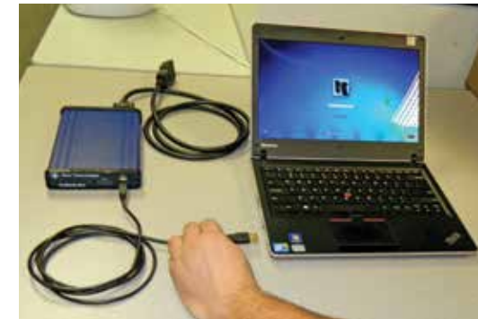
The SAE J2534 device cable plugs into PC and under-dash OBD II connector.
