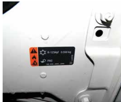
Label on Cadillac ATS says it's R-1234yf equipped. Note flame symbol in orange section at left. (Paul Weissler)
