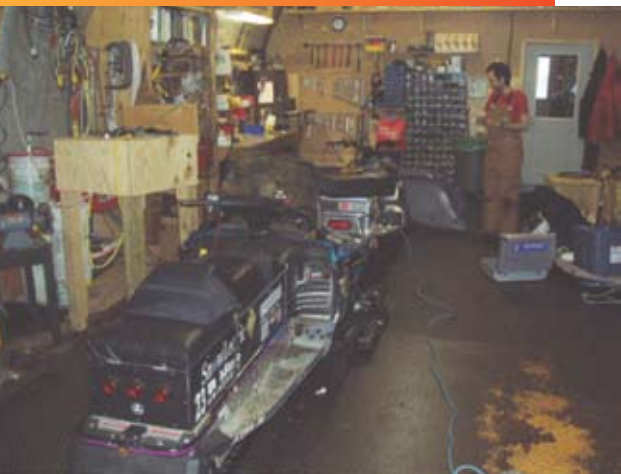
Both electric snowmobiles in the shop at Summit Station. Machines had to be equipped with electric heaters, and optimized for use in the polar environment.
