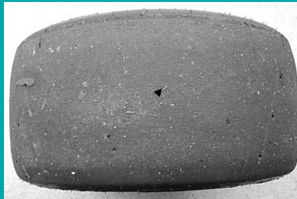
Example of good tire wear, small grain pattern and even wear across full tread arc
