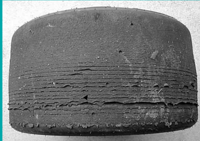
Insufficient camber gain in roll, too little static camber
