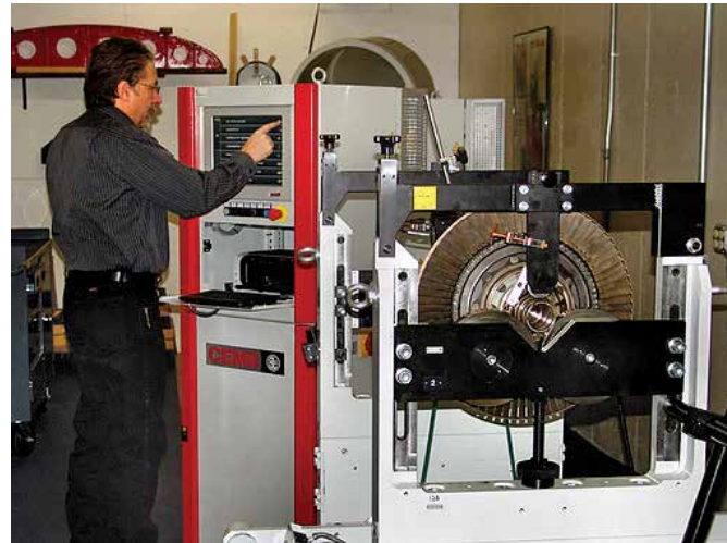
A jet engine is balanced at the Vibration Solutions North Rotor
