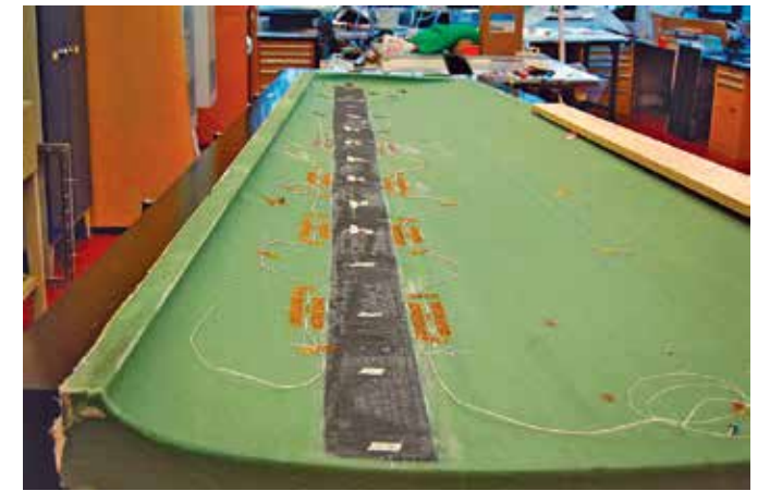
Intelligent load-monitoring sensor technologies are being developed to detect or calculate the residual fatigue life and structural health of a composite wing. (Fraunhofer Institute)
