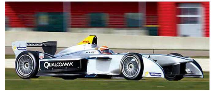
The Spark-Renault sRT_01E is the racecar used by all teams in the new all-electric Formula E series.
