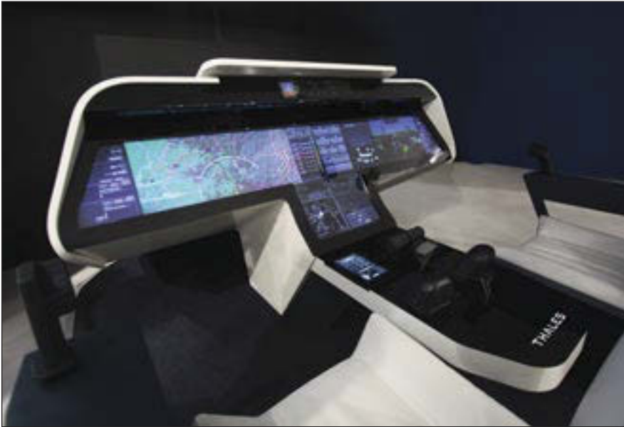
Thales supplies all the cockpits and flight control systems for the Airbus family. This is ODICIS, a futuristic concept for a wrap-around display system incorporating the latest apps technology and maximum display flexibility.
