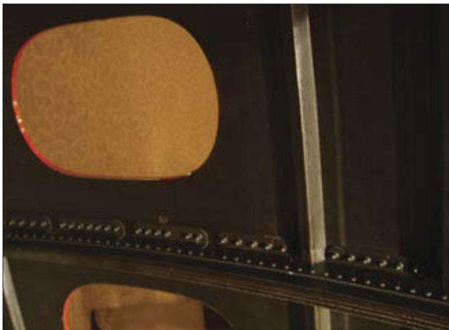
Closeup of a 787 fuselage panel showing the composite structure with metal fasteners and strengtheners. (Richard Gardner)
