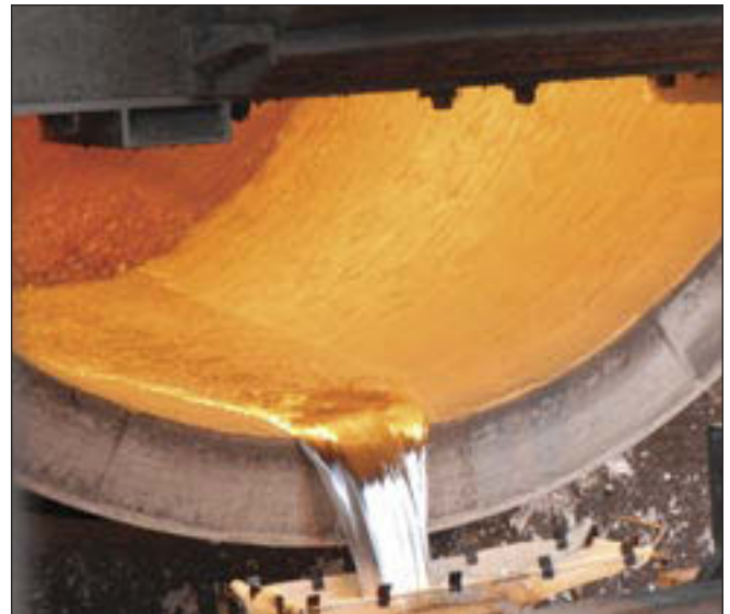
At its Issoire recycling casthouse, Constellium has demonstrated the recyclability of A300 wings and cockpit parts with a recovery yield of over 90%, resulting in new aluminum ready for use in future aircraft.
