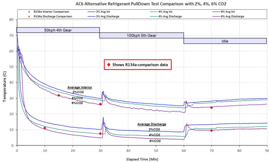
Figure A: pulldown curves for varying composition of AC6
