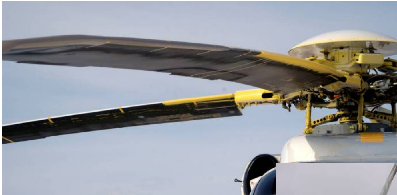
Main Rotor After Failure Simulation in Artificial Icing
